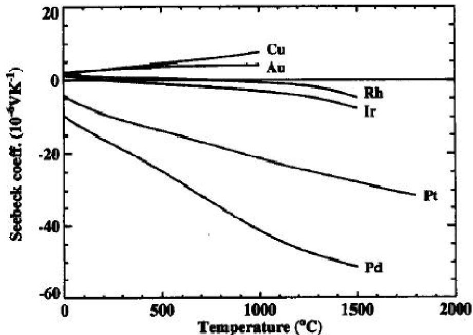
Fig. 1 - Seebeck coefficients of different elements derived from the relative rates of Pt, data EMS / and the absolute temperature coefficient for Pt.
