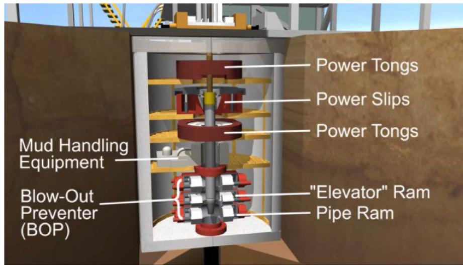
**Figure 5. Shielded "basement" equipment for handling waste packages.**
