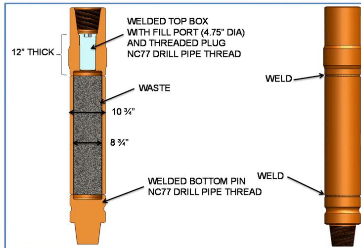
**Figure 3. 27.3-cm (10.75-inch) OD flask-type design, aspect ratio shortened for illustration (Su and Hardin 2015)**
