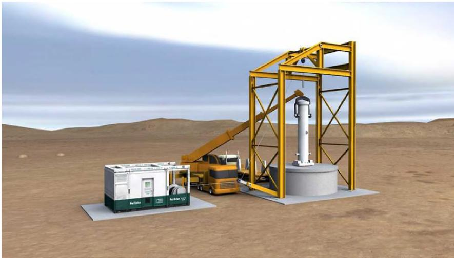
**Figure 6 wireline handling and emplacement components.**
