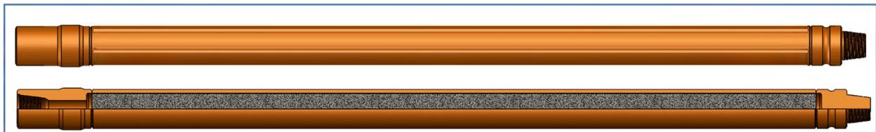
**Figure 4. 27.3-inch OD flask-type design, shown at true aspect ratio (Su and Hardin 2015)**
