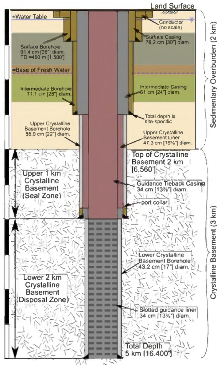
**Figure 2 DBFT Conceptual Design (Kuhlman, K.L., et al, 2015)**
