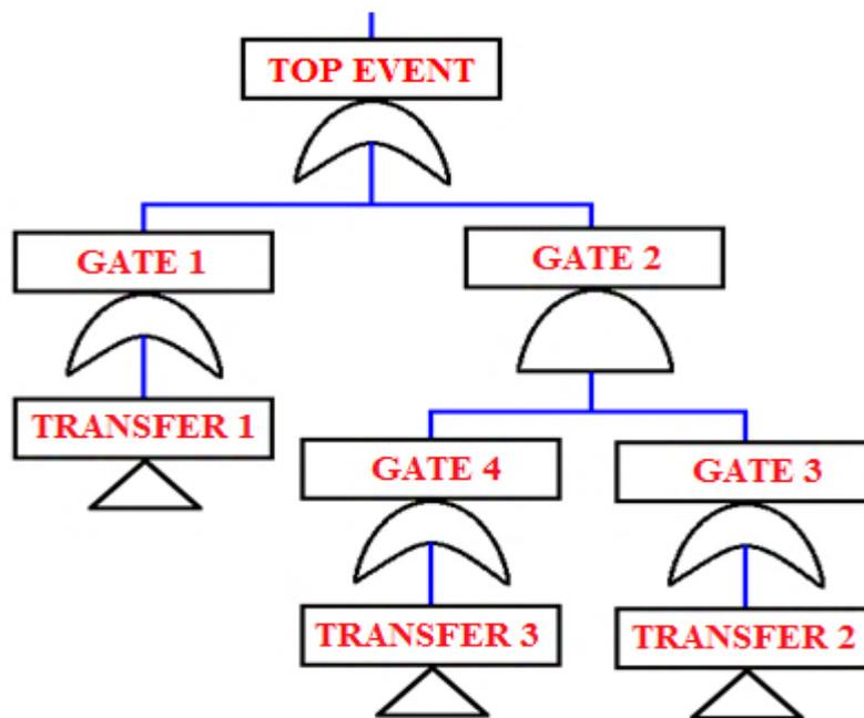
Figure 4. Main Fault Tree of CSIS [7].
