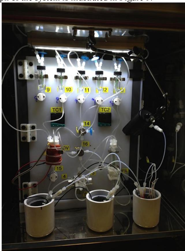
**Figure 5. Photograph of the  $^{86}\text{Y}$  automated purification system. Irradiated  $^{86}\text{SrO}$  targets are dissolved in the heated dissolution vessel (above valve 15). The liquid is pH adjusted and then transferred over the filter paper (FIL). By manipulating the pH of the solutions, the Sr target material can be separated from the  $^{86}\text{Y}$  product.**
