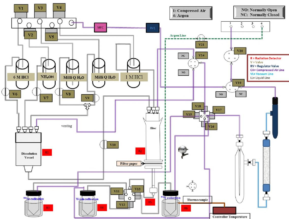
**Figure 4. Schematic of the  $^{86}\text{Y}$  automated purification system. Irradiated  $^{86}\text{SrO}$  targets are dissolved in the dissolution vessel. The liquid is pH adjusted and then transferred over the filter paper. By manipulating the pH of the solutions, the Sr target material can be separated from the  $^{86}\text{Y}$  product.**
