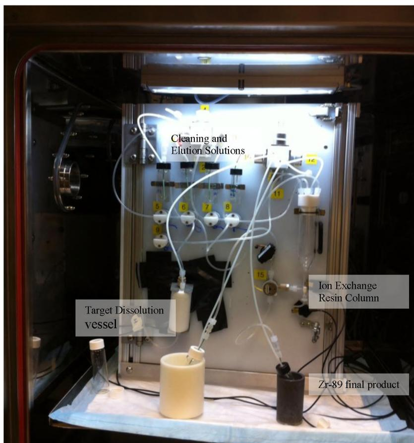
**Figure 1. Washington University Zr-89 purification system**
