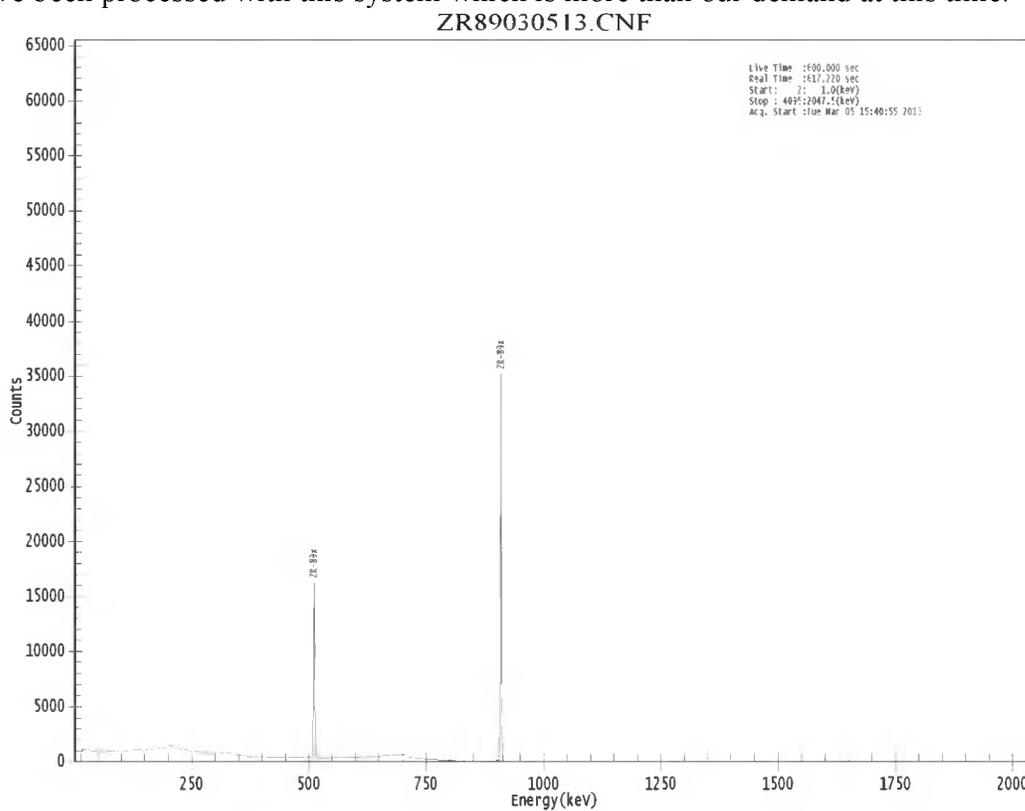
**Figure 2. Gamma Ray spectrum of <sup>89</sup>Zr produced on March 5<sup>th</sup>, 2013. Note peaks at 511 keV (positron annihilation peaks) and 909 keV (signature gamma ray from <sup>89</sup>Zr)**
