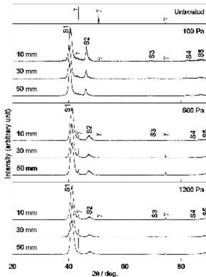
Figure 1. XRD pattern of AISI 304 steel sample treated at 723 K by ASPN.
