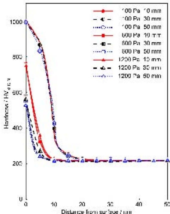
Figure 5. Hardness distribution from surface of AISI 304 steel sample treated at 723 K by ASPN.
