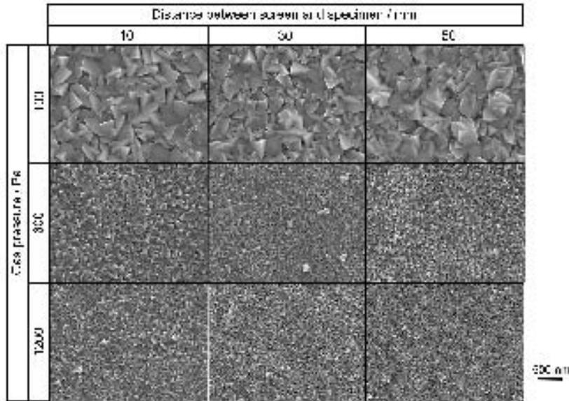
Figure 2. SEM micrographs of AISI 304 steel sample treated at 723 K by ASPN.
