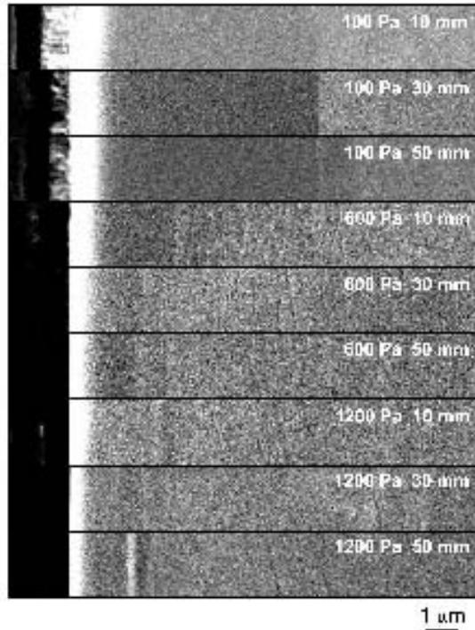
Figure 3. Cross sectional microstructures of AISI 304 steel sample treated at 723 K by ASPN.
