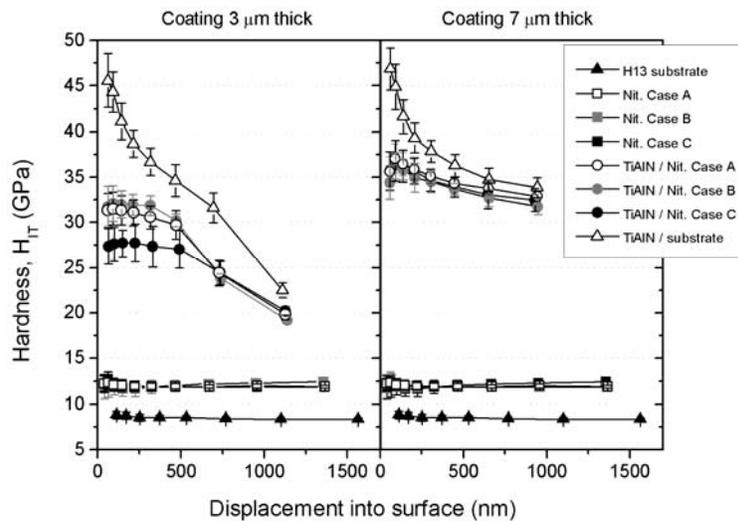
Figure 5. Instrumented Hardness of nitrided and non nitrided AISI H13 coated with TiAlN.
