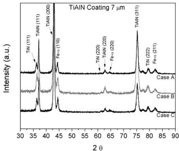
Figure 4. XRD patterns of the coating with thickness of 7 μm deposited over nitrided cases A, B and C.
