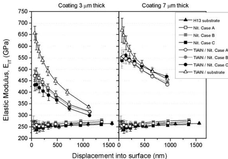
Figure 6. Elastic modulus of nitrided and non nitrided AISI H13 coated with TiAlN.
