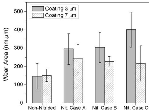
**Figure 7.** Worn area of nitrided and non nitrided AISI H13 coated with TiAlN.
