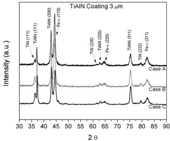
Figure 3. XRD patterns of the coating with thickness of 3 μm deposited over nitrided cases A, B and C.
