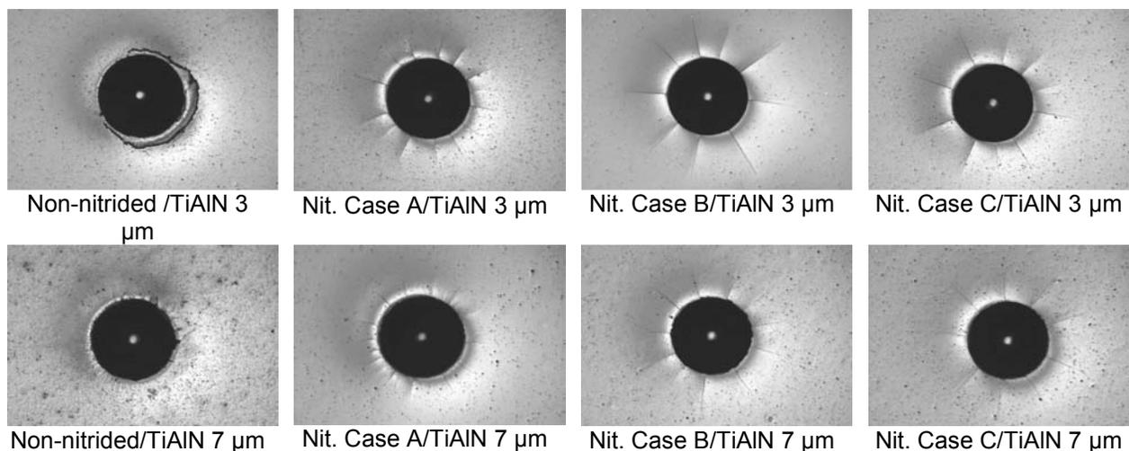
**Figure 8.** Rockwell C indentation aspect of nitrided and non nitrided AISI H13 coated with TiAlN.
