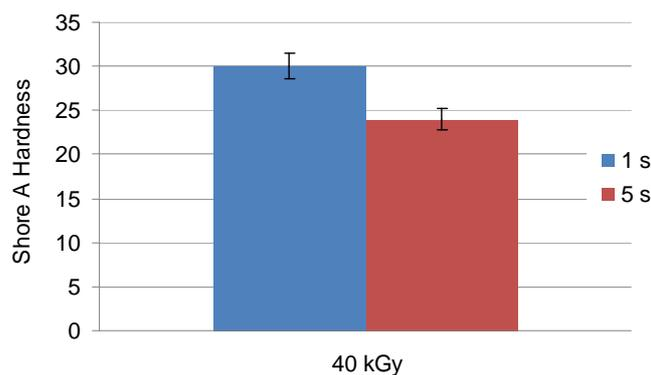
Figure 1: Shore A hardness of composite containing 10% Brazil nut shell fiber, electron beam irradiated with a dose of 40 kGy.
