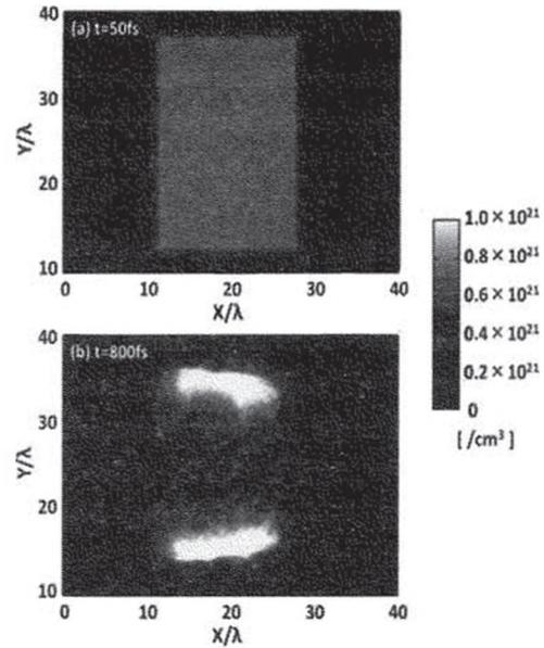
Fig. 7 Electron density of the plasma target, after the laser passed through the target
