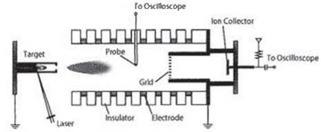
Figure 4: Cross-sectional diagram of electrodes.
