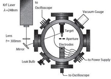
Figure 3: Schematic drawing of the experimental apparatus.
