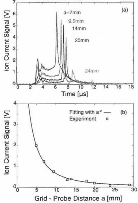
(a) Ion current signals at  $a = 7 \sim 24$ mm when 300 V is applied to the control electrode
