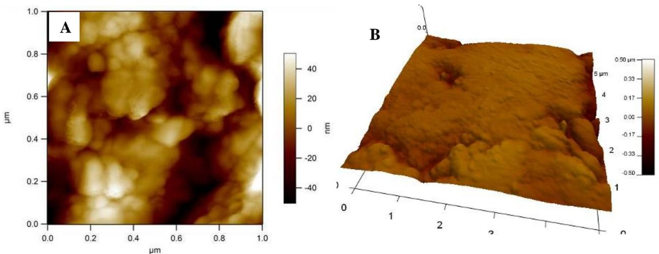
Figure 5 – Micrographs: A) the microtopographic profile of the region near the roughcast mortar/mortar plastering interface, B) 3D topographic profile of the same region.
