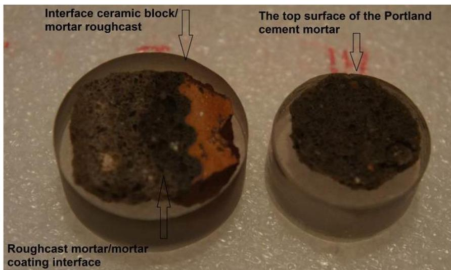
Figure 1 – Portland cement mortar samples prepared for AFM.
