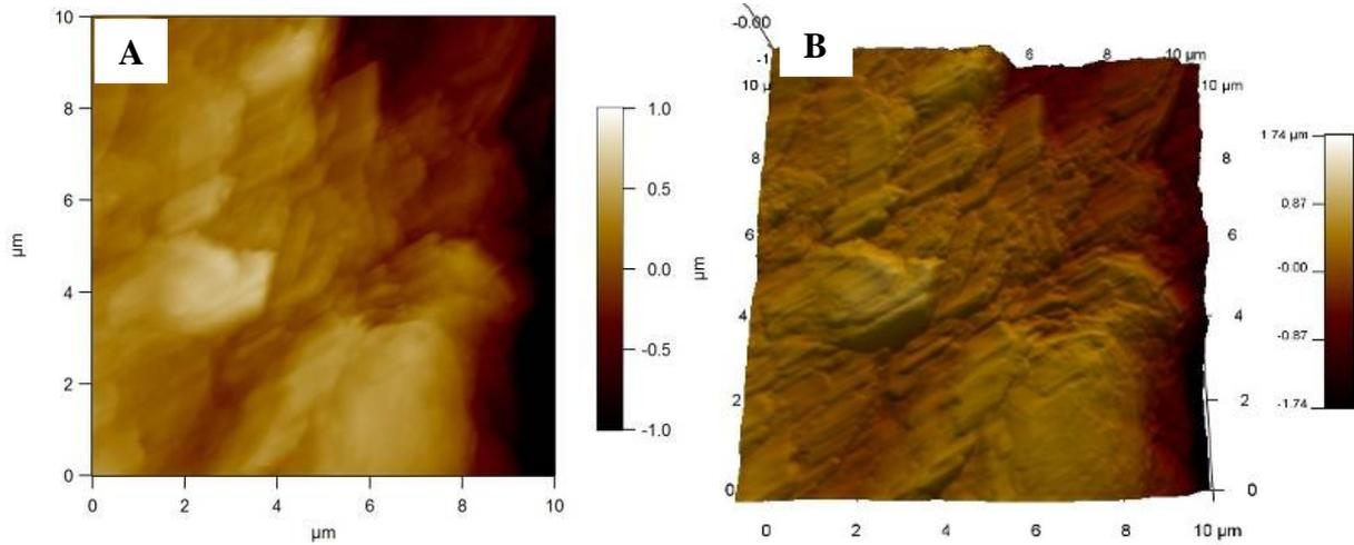
Figure 4 – Micrographs: A) the microtopographic profile of the region close to the ceramic block/mortar interface; B) 3D topographic profile of the same region.
