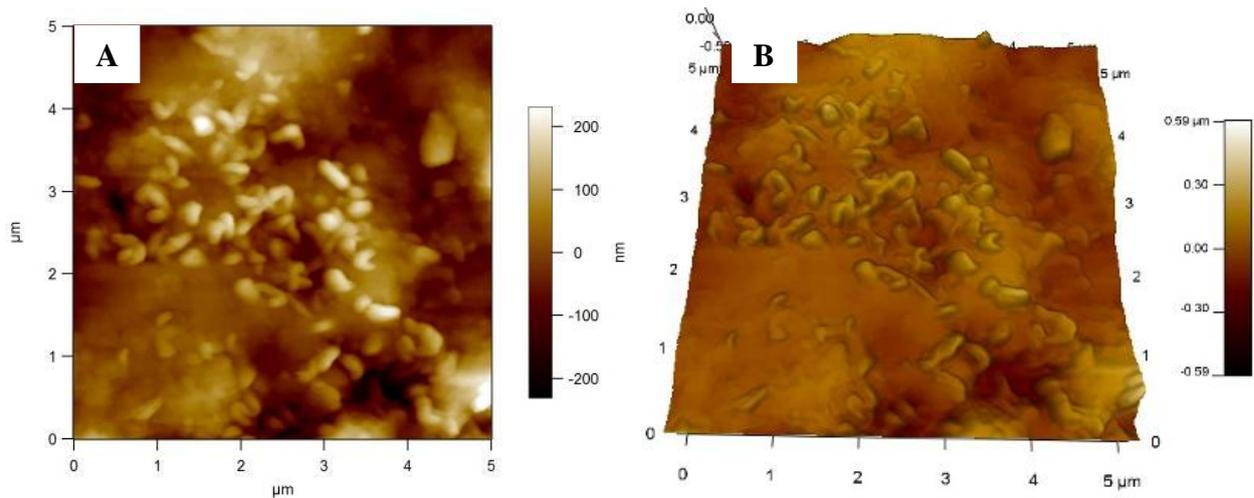
Figure 3 – Micrographs: A) the microtopographic profile of the region close to the ceramic block/mortar interface; B) 3D topographic profile of the region close to the ceramic block/mortar interface.
