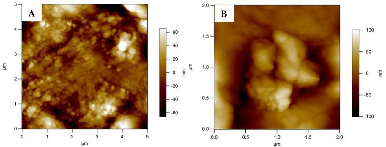
Figure 2 – Micrographs of the microtopographic profile of the region close to the ceramic block/mortar interface.
