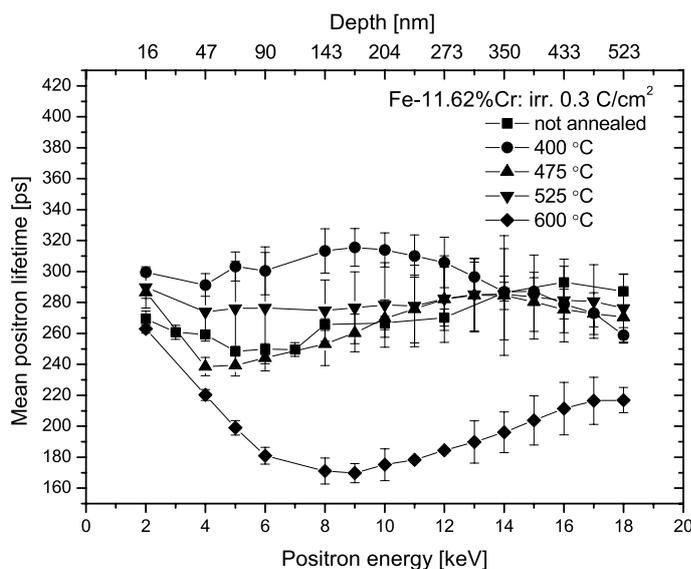
Fig.1: Mean positron lifetimes of annealed Fe-11.62%Cr alloys.
