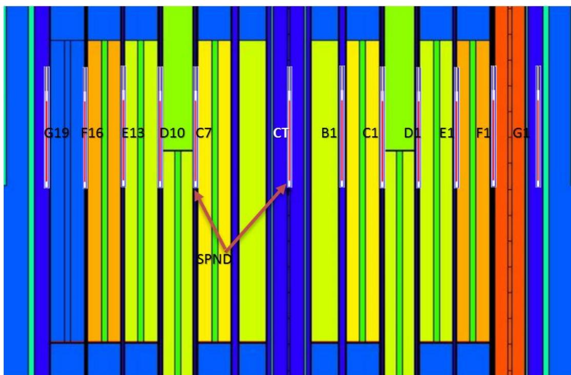
Figure 4, Side view of RTP core model in with actual control rod position during the measurement.
