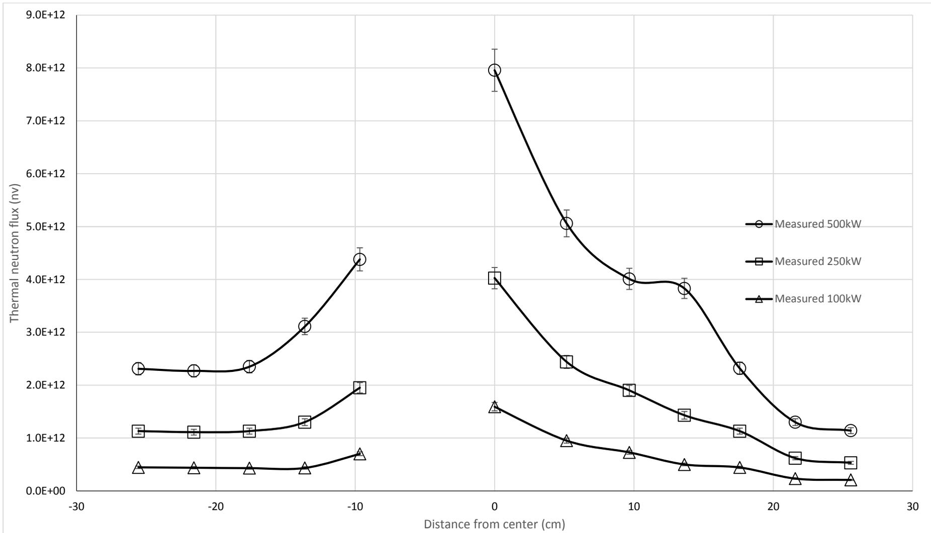
Measurement results of in-core thermal flux profile at 100 kW, 250 kW and 500 kW
