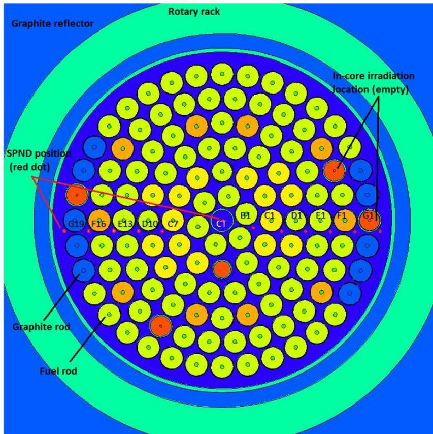
Figure 5, Top view of RTP core showing SPND position.
