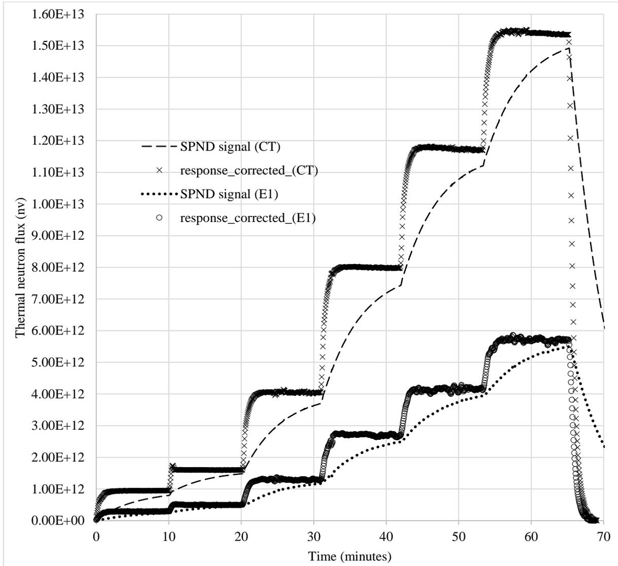
Figure 7, Gradual increase of thermal neutron flux measurement at Central Thimble (CT) and E1 for gradual increase of core power level from zero power to maximum 1 MW.
