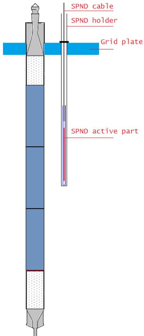
Figure 3, Schematic diagram of RTP fuel with SPND inserted in a holder which left hanging on the top of core grid plate where the axial position can be adjust.
