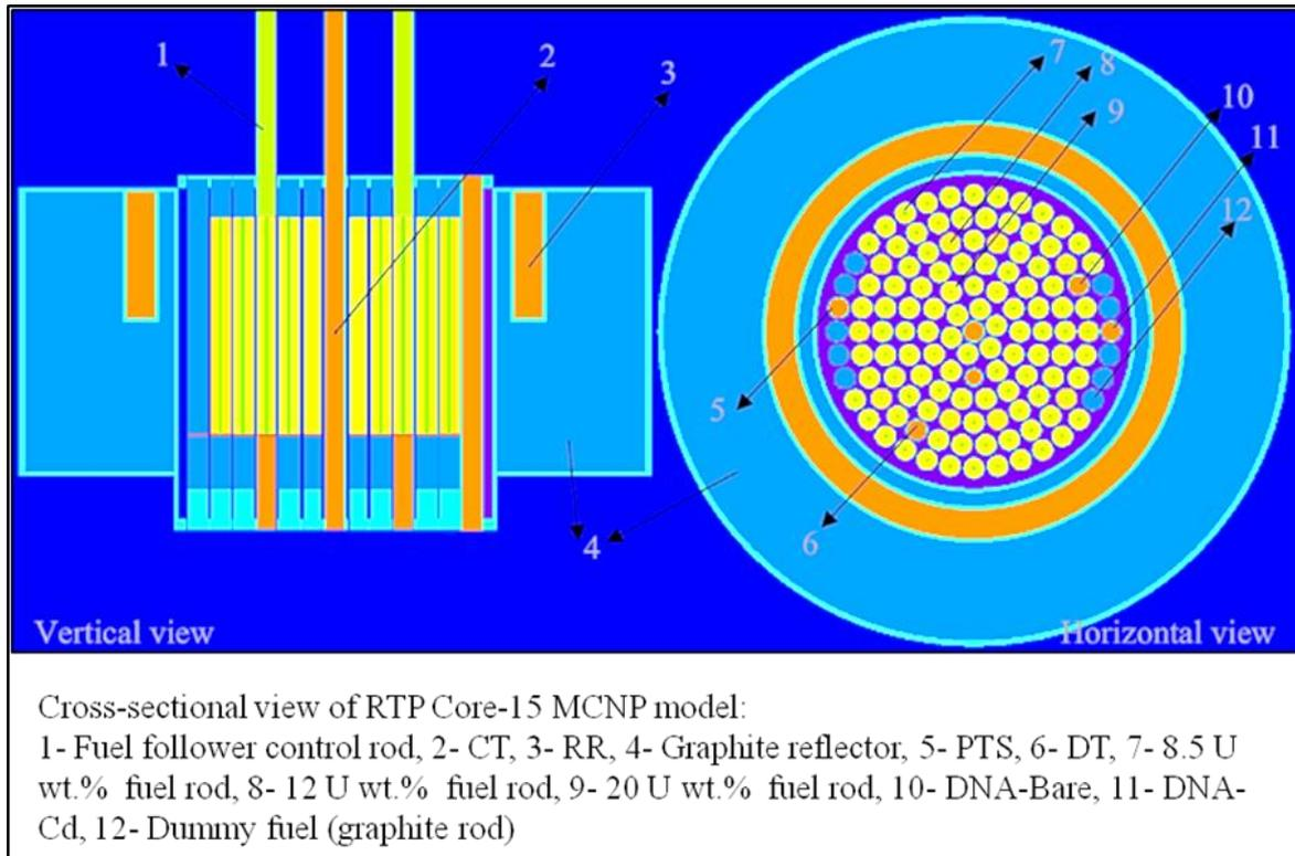
Figure 1, Side and top view of RTP Core-15 configuration.
