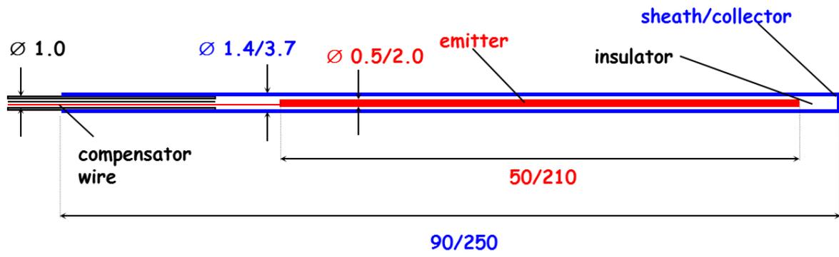
Figure 2, Schematic diagram of sensitive region of SPND used in RTP.
