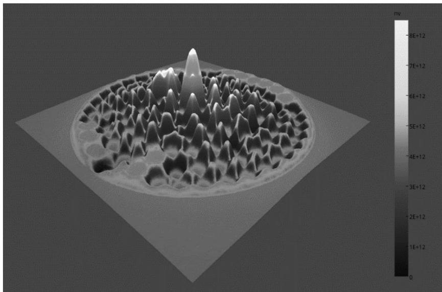
Figure 6, Thermal neutron flux distribution inside RTP core predicted by MCNP simulation where the maximum flux located at the centre of the core (in Central Thimble irradiation facility). The maximum thermal flux value is around  $8.7 \times 10^{12} \text{ n}\cdot\text{cm}^{-2}\cdot\text{s}^{-1}$  at 500 kW core power level.
