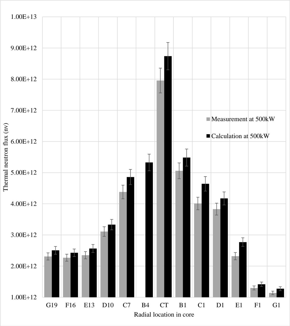
Figure 8, Comparison between calculated and measured in-core thermal neutron flux.
