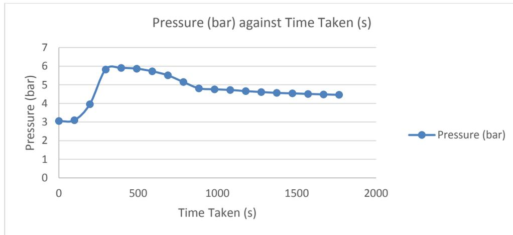
Figure 7: Correlation between pressure and time for oil sludge sample
