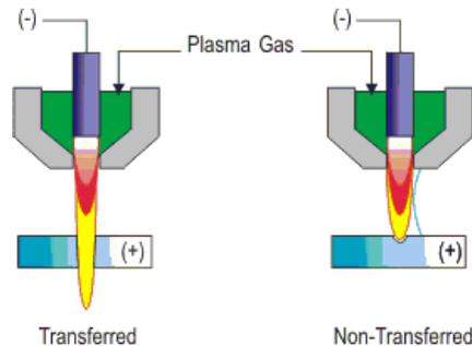
Figure 1: Comparison transferred and non-transferred arc torch
