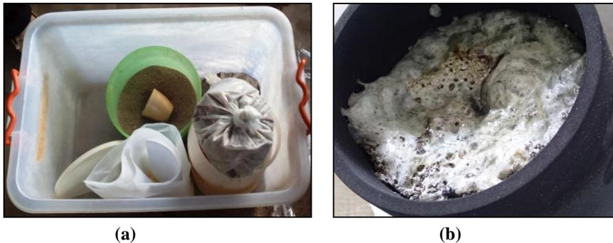
Figure 5: (a) The sample of oil sludge change to partial immobilization glass after running about 12 minutes (b) The oil sludge and sand samples after plasma testing
