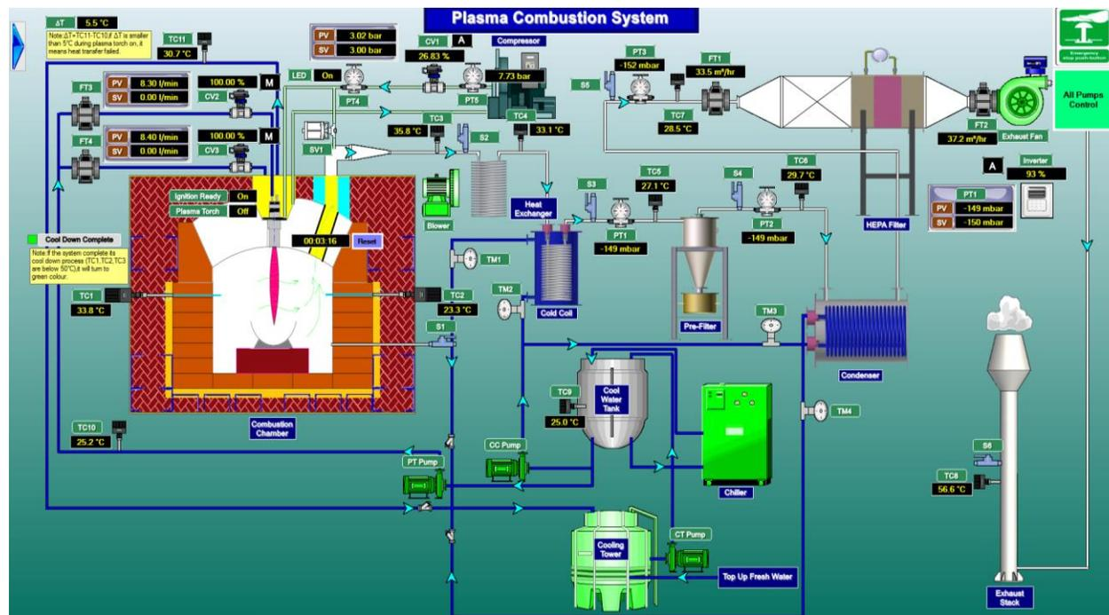
Figure 3: Thermal Plasma Pilot Plant Process
