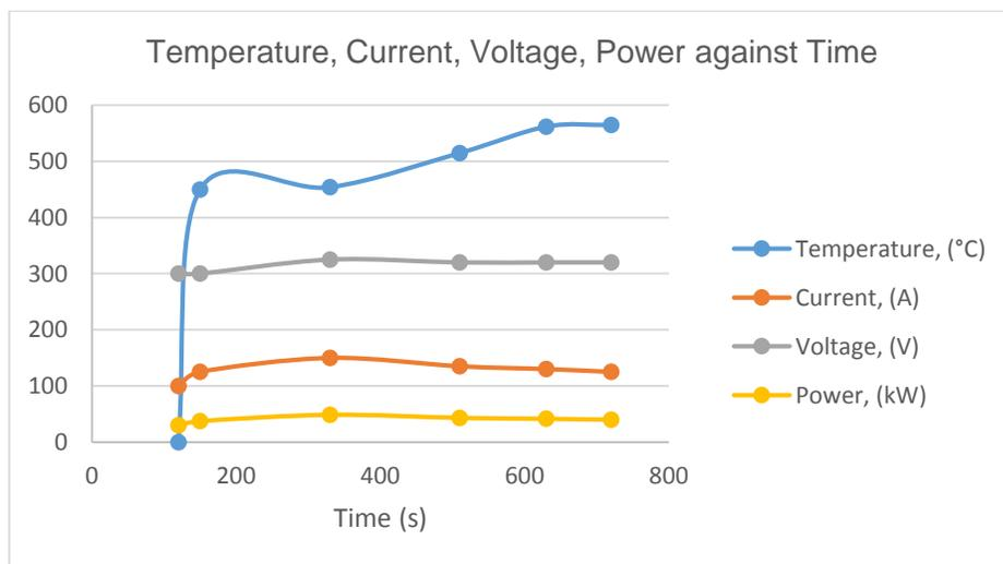
Figure 6: Correlation between temperature, voltage and current with time for oil sludge sample
