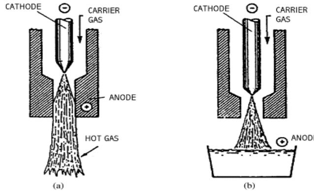
Figure 2: Different between transferred arc torch (a) and non-transferred arc torch (b) of plasma.
