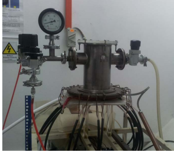
Figure 2: Plasma focus device at Nuclear Malaysia Agency
