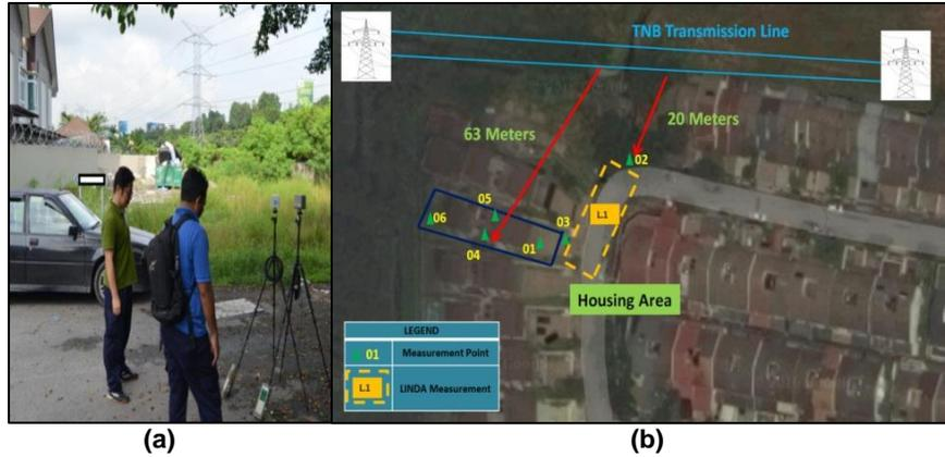
Figure 2: (a) Setup of equipment and (b) layout of the measurement point locations for Case TL2
