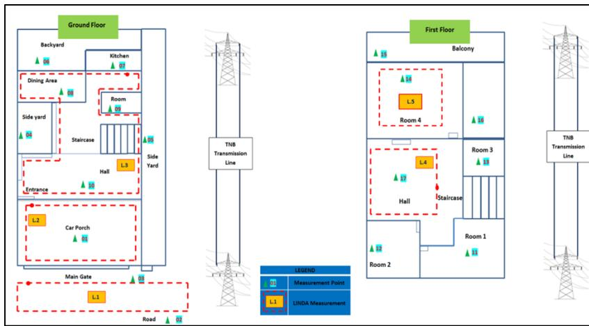
Figure 3: Layout of the measurement point locations inside the house for Case TL2
