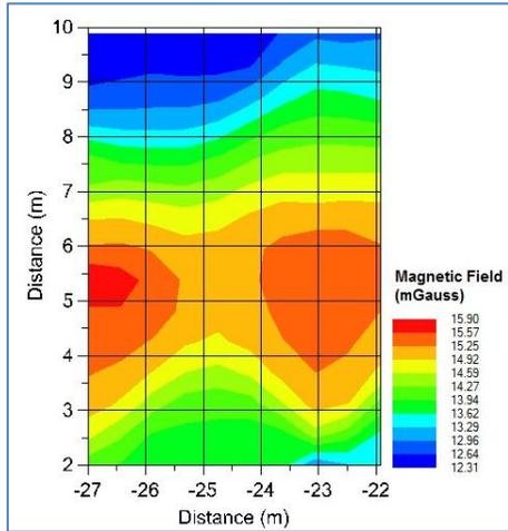
Figure 9: Contour map of magnetic field strengths at location L.1 (case TL3)
