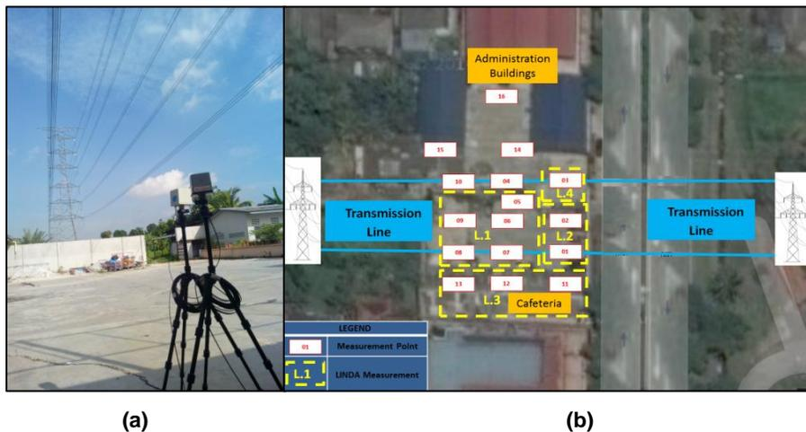
Figure 4: (a) Setup of equipment and (b) layout of the measurement point locations for Case TL3
