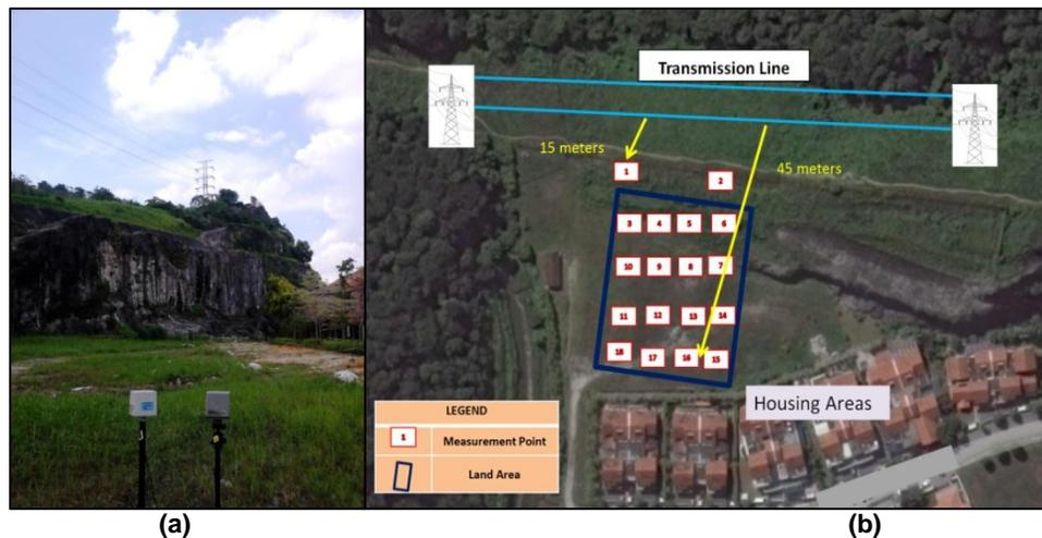
Figure 1: (a) Setup of equipment and (b) layout of the measurement point locations for Case TL1
