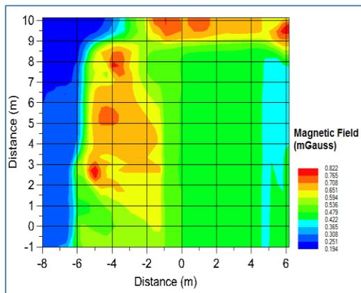
Figure 7: Contour map of magnetic field strengths at location L.1 (case TL2)
