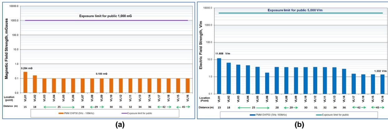
Figure 5: Plot of ELF (a) magnetic field strength and (b) electric field strength against distance and point of measurement and their comparison with the public exposure limits
