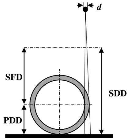
Figure 2: Test arrangement and distances for tangential radiography with the source offset from the pipe centre line
