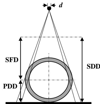
Figure 1: Test arrangement and distances for tangential radiography with the source located on the pipe centre line
