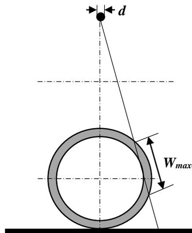
Figure 3: Maximum penetrated thickness,  $W_{max}$ , for the tangential radiography technique
