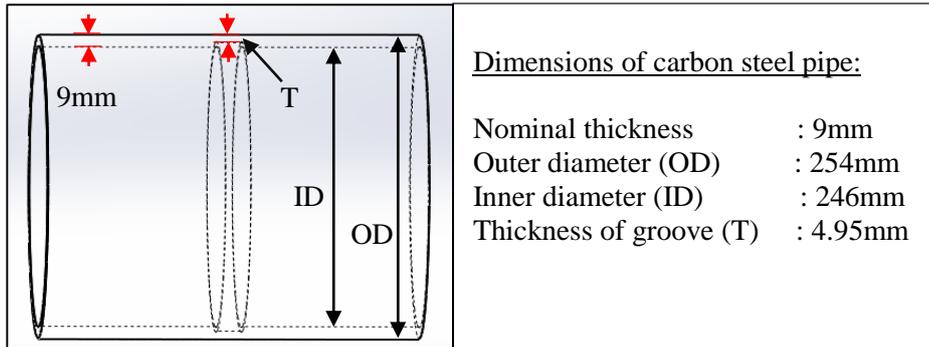
Figure 4: Schematic diagram of the pipe
