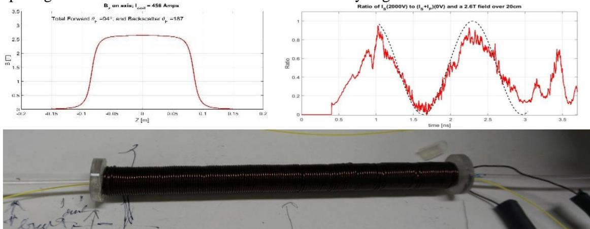
Fig 8 8a) The simulation of the field in the solenoid shown in 8c), 8b) the reconstructed Faraday rotation from the new Backscatter Tailored optical fiber with a dotted trace the expected curve for the 2.6T solenoidal field. The position matches very well indicating the spatial dependence of the field is captured as indicated by the dotted curve, 8c) shows the 20cm long solenoid with the fiber threading the bore.
