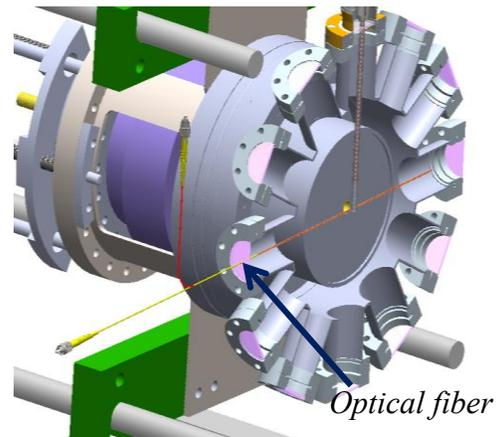
**Fig 2** Shock chamber with a fiber sensor across the bow of the magnet.
