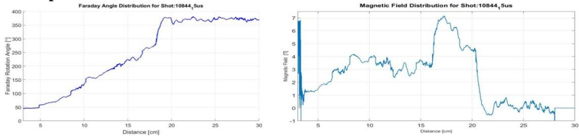
**Fig 9** Fiber optic pulsed polarimetry traces for shot 10844 showing a 7T peak field in front of the magnet surface. 9a) progressive Faraday rotation along fiber, 9b) the derivative of 9a) or local B field along the fiber.
