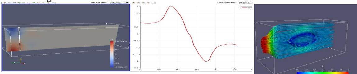
**Fig. 7c)** Shows simulations of translating FRC impacting the stagnating magnetic field. 7 a,b) are the radially directed magnetic field profile of the FRC in front of the magnet. The MSX geometry is fully represented.
