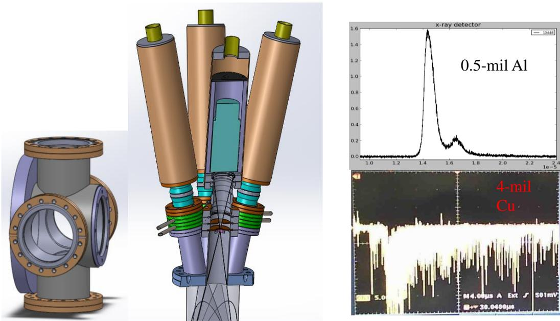
**Fig 6** Some of the changes to MSX and diagnostic structures that were implemented on this short time scale, Swks cad drawings show a) the new shock chamber, b) a multi-foil X-ray detection system and c) initial X-ray signals which show copious amounts of hard X-rays.
