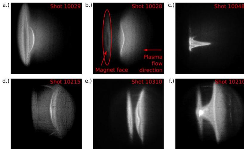
**Fig 5** Top row – Mirror field + gas puff: a.) weak, b.) intermediate, c.) strong field. Bottom row – cusp field + gas puff: d.) weak, e.) intermediate, f.) strong.
