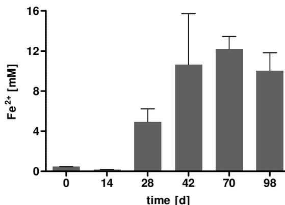
Fig. 1: Microbial influence on  $Fe^{2+}$ -concentration within the Bentonite B36. Iron determination was carried out according to a modified Ferrozine-method based on Viollier *et al.*<sup>[1]</sup> Shown are mean values with standard deviations from at least two independent experiments conducted in duplicates.
