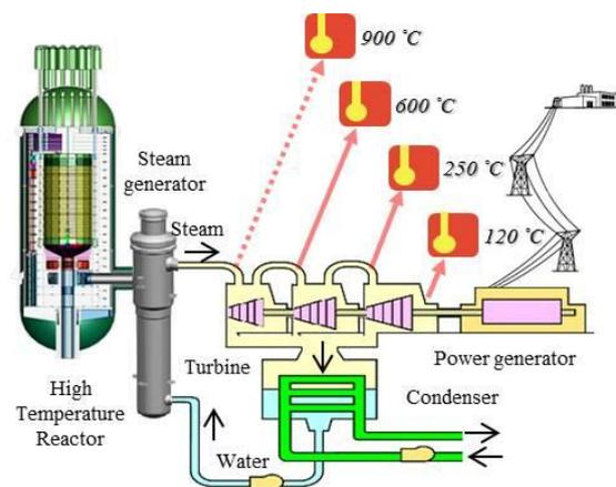
Fig. 2: Illustration of the expected cogeneration capabilities of HTRs
