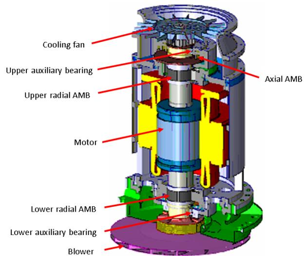
Figure 4. The structure and picture of the helium blower rig
