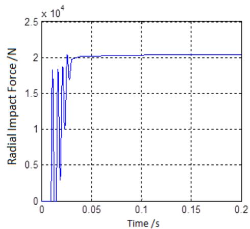
Figure 7. Radial impact force curve of the dropping rotor
