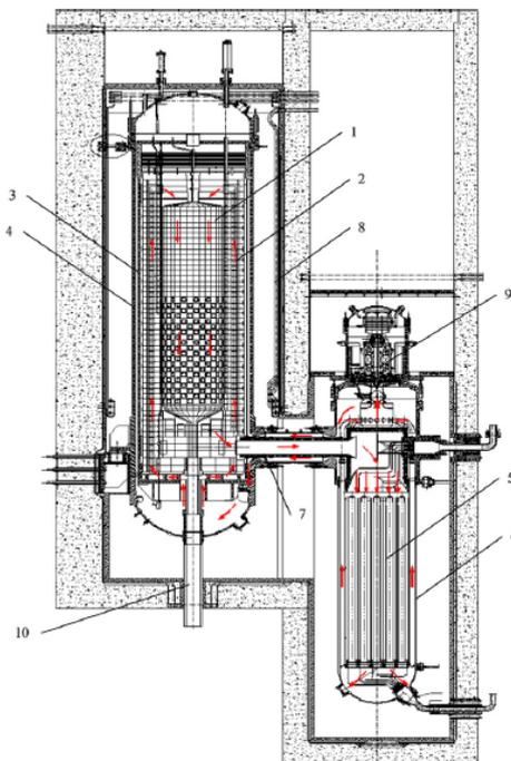
Fig. 1. Cross section of the primary circuit of the HTR-PM. 1, reactor core; 2, side reflector and carbon thermal shield; 3, core barrel; 4, reactor pressure vessel; 5, steam generator; 6, steam generator vessel; 7, coaxial gas duct; 8, water-cooling panel; 9, blower; 10, fuel discharging tube
