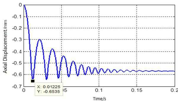
Figure 5. Axial displacement curve of the dropping rotor
