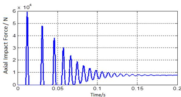
Figure 6. Axial impact force curve of the dropping rotor
