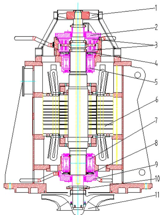
Fig. 2. Structural components of the blower. 1, cooling fan; 2, upper auxiliary bearing; 3, axial AMB; 4, upper position sensor; 5, upper radial AMB; 6, electric motor; 7, lower radial AMB; 8, lower position sensor; 9, lower auxiliary bearing; 10, rotor; 11, blower wheel
