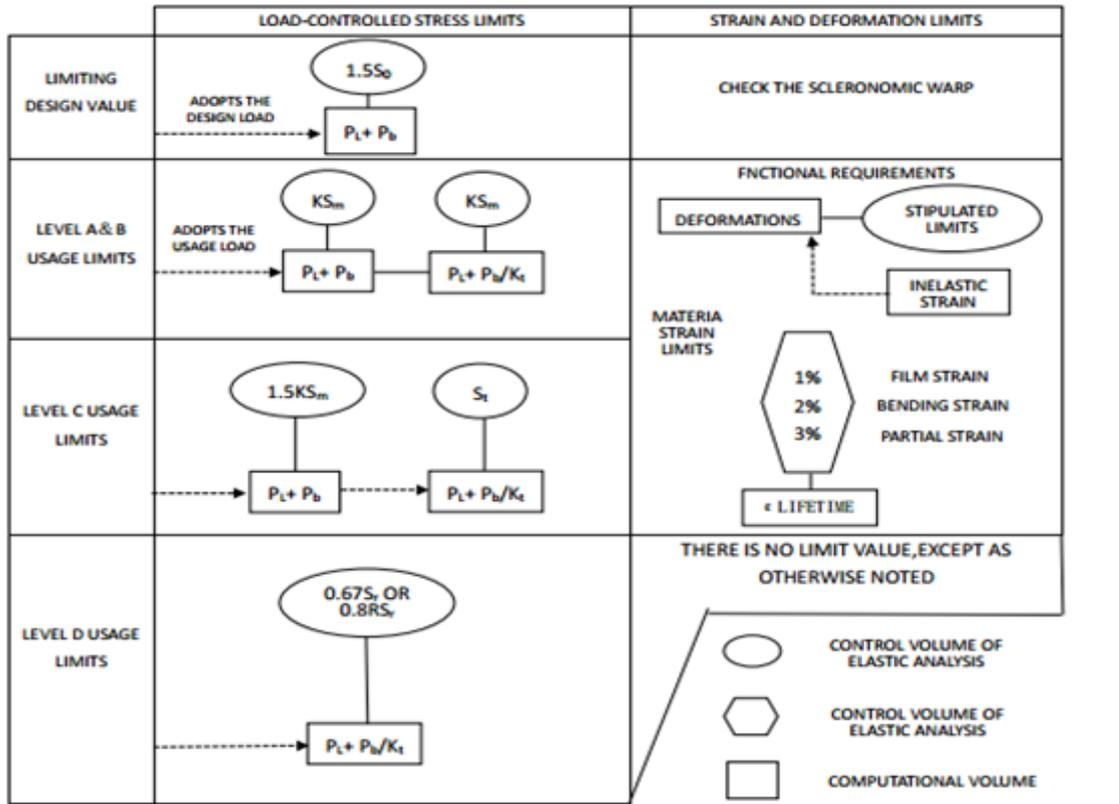
Fig 1: Flow diagram for high temperature design
