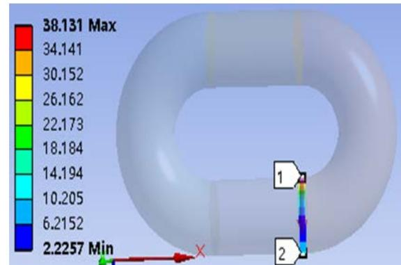
Fig 3: Linearized stress intensity
