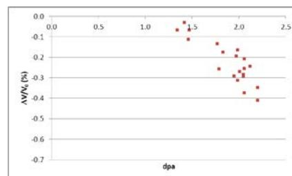
Fig. 4: Low Dose Test: Dimensional Change against Neutron Fluence for Graphite irradiated at 750°C
