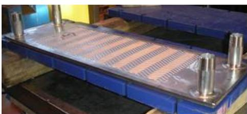
Fig. 5: Stainless steel mockup to check CFD thermal and Hydraulic laws
