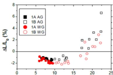
Fig. 3: Dimensional Change tests against levels of Neutron Fluence for a Graphite sample irradiated at 750°C
