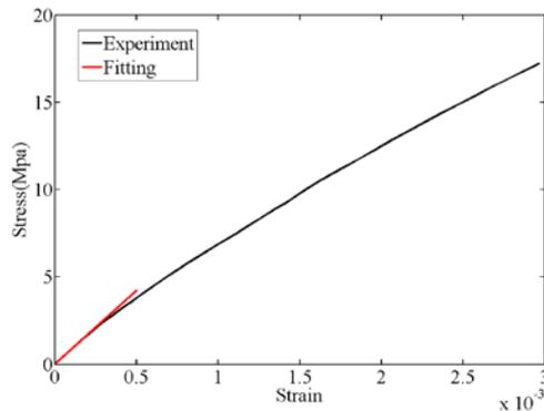
Fig. 11. The average stress-strain curve and the fitting line of the elastic modulus during the period of elasticity
