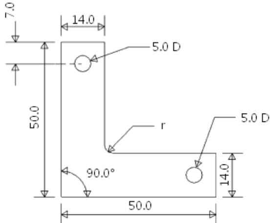
Fig. 1. Dimensions of L-shaped sample (in mm)
