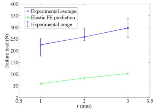
Fig. 7. The comparison results of numerical simulation and experimental results on maximum fracture load
