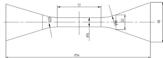
Fig. 8. The dimensions of the specimen (in mm)
