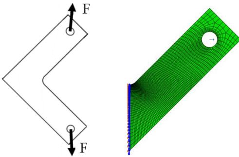
Fig. 6. The finite element model of L-shaped specimen
