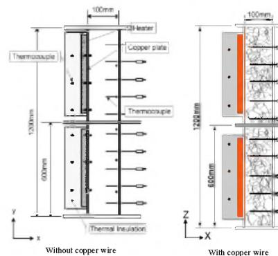
Fig.2 Experimental apparatus ((a) without copper wire, (b) with copper wire)
