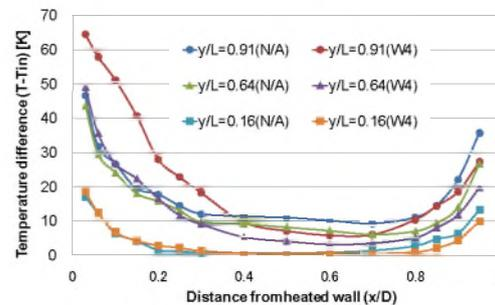
Fig.7 Distribution of gas temperature along the channel width (736W, W4&N/A)
