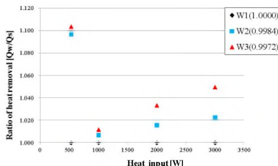
Fig. 24 Thermal performance of rectangular channel inserting porous material
