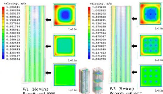
Fig.18 Flow velocity of air (Left: no wire, Right: 9 wires)
