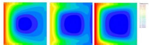
Fig.12 Temperature distribution of air (Left: outlet, Center: center, Right: inlet)
