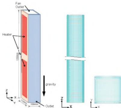
Fig.11 Analytical model of the vertical rectangular channel
