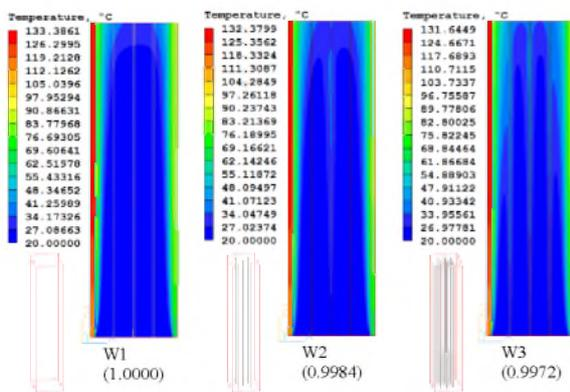
Fig.20 Temperature distribution of air at Y-plane (529W)
