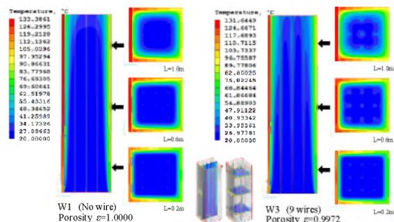
Fig. 17 Temperature distribution of air (Left: no wire, Right: 9 wires)
