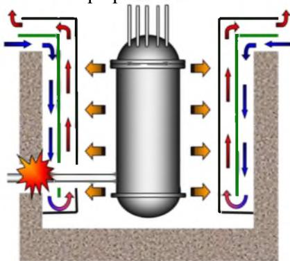
Fig.1 Schematic drawing of passive cooling system
