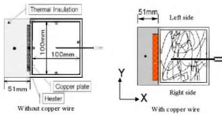
Fig.3 Cross section ((a) without copper wire, (b) with copper wire)
