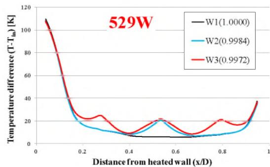
Fig.22 Temperature distribution of air along the channel width
