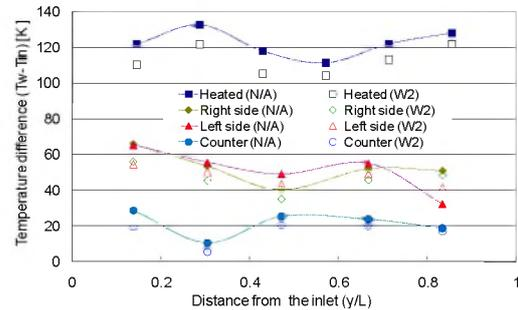
Fig. 8 Distribution of wall temperature along the flow direction (736W, W2&N/A)
