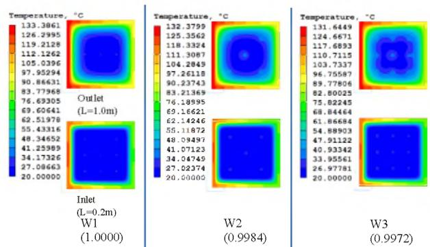
Fig.21 Temperature distribution of air at Z-plane (529W)
