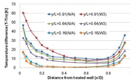
Fig.6 Distribution of gas temperature along the channel width (736W, W3&N/A)
