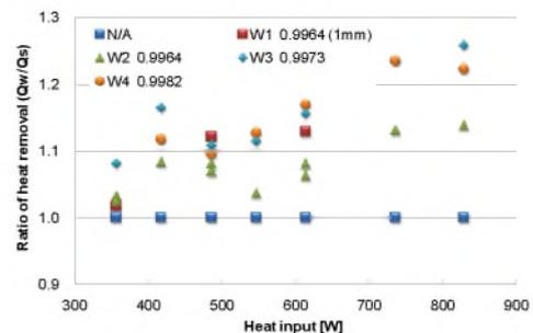
Fig. 10 Thermal performance of rectangular channel inserting porous material
