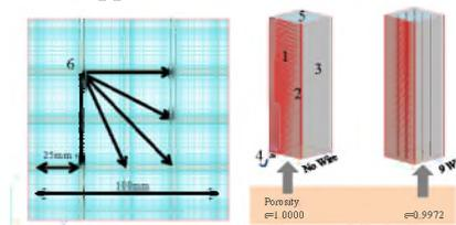
Fig. 16 Analytical model of the vertical rectangular channel inserting the copper wire
