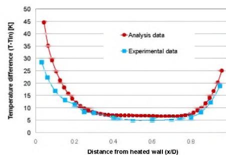
Fig.13 Temperature distribution of air along the channel width
