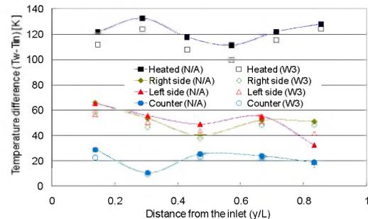
Fig. 9 Distribution of wall temperature along the flow direction (736W, W3&N/A)
