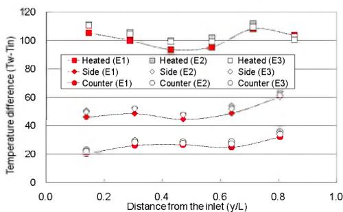
Fig. 14 Temperature distribution of wall along the flow direction (E1&E2&E3)
