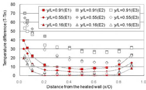
Fig. 15 Temperature distribution of air along the channel width (E1&E2&E3)
