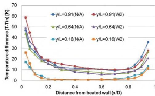
Fig.5 Distribution of gas temperature along the channel width (736W, W2&N/A)
