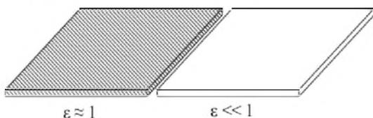
Fig. 3: Heat flux sensor pairs. Black matte (left), shiny reflective (right)
