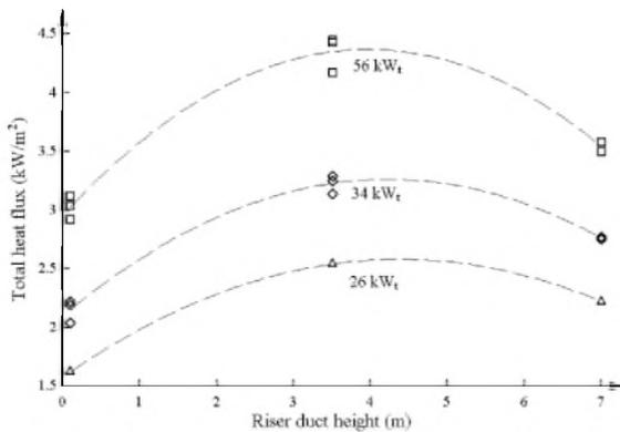
Fig. 6: Heat flux (hot riser face) for varying powers
