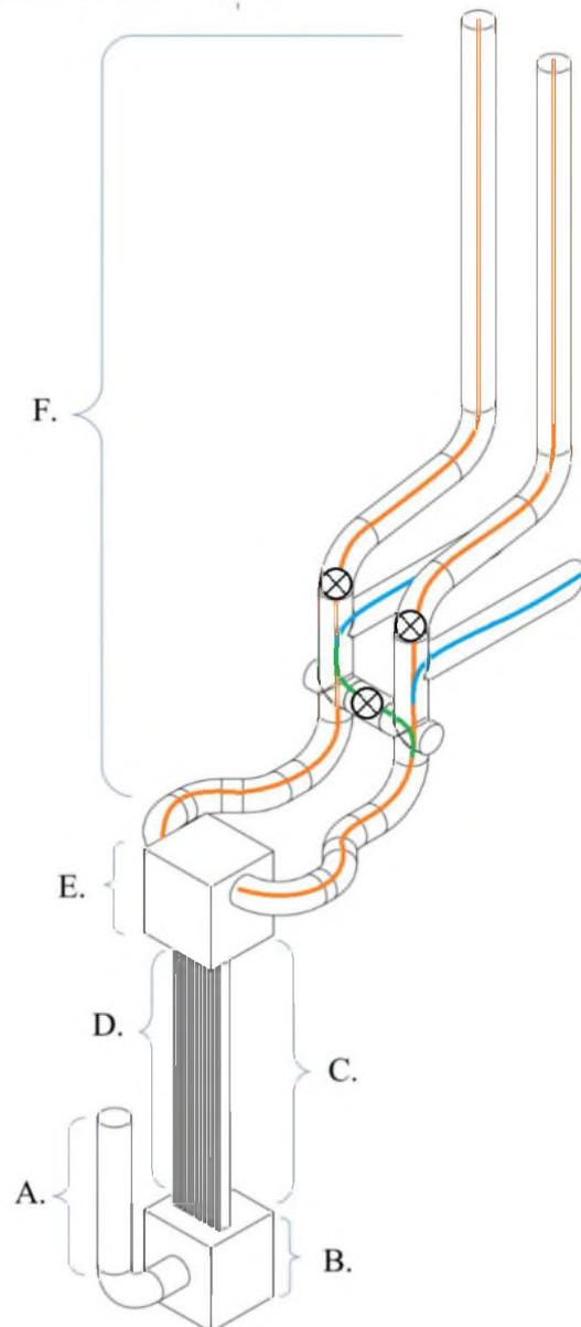
Figure 2: Simplified model of 1/2 scale NSTF. A. inlet downcomer, B. inlet plenum, C. heated cavity, D. riser tubes, E. outlet plenum, F. chimney. Flow paths for varying chimney roles: Baseline (orange), reduced discharge (blue), single chimney (green). Crossed circles represent manual valves.
