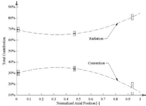
Fig. 5: Heat flux distribution from heated plate to front surface of riser ducts, baseline case
