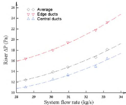
Fig. 8: Riser ΔP vs. system mass flow, baseline configuration at varying integral powers
