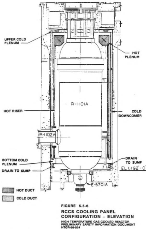
Fig. 1: GA-MHTGR RCCS concept [2]
