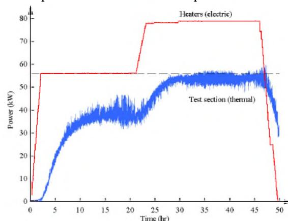
Fig. 4: Electric and thermal powers for baseline test case, dual vertical chimney exhaust
