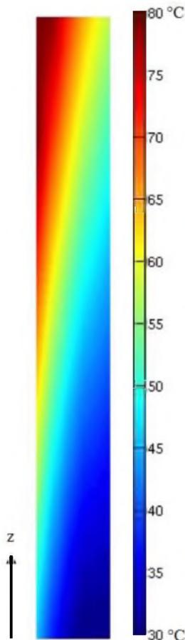
Fig. 13: 2D contour map of gas space temperatures, generated from five LUNA fiber cables along full length of riser duct at baseline test conditions
