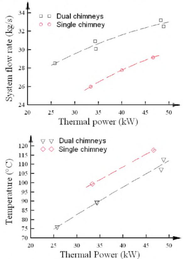
Fig. 11. System parameter trends for varying chimney configurations.
