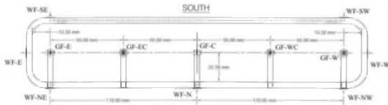
Fig. 12: Position of LUNA fibers in NSTF
