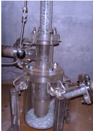
Fig. 5: Typical photograph of flow pattern of the feeder and the bottom of the riser for steady conveying at high u_a .
