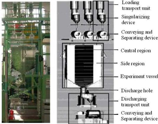
Fig. 1: Pebble flow experiment rig in INET.
