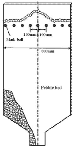
Fig. 2: The quantitative experimental method of pebble flow.
