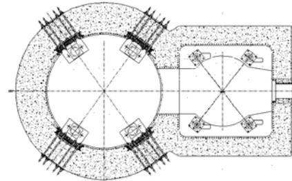
Fig.3 Diagram of main equipment support in primary loop cavity
