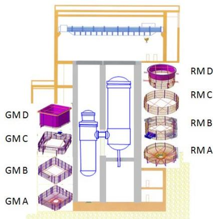
Fig.4 Diagram of modular design scheme of primary loop cavity
