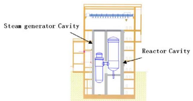
Fig.1 Section view of primary loop cavity of HTR-PM
