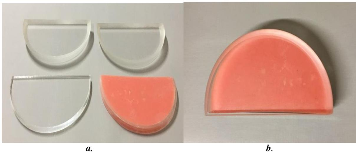
**Figure 3: Breast phantom. Plates (a) and assembled (b).**
