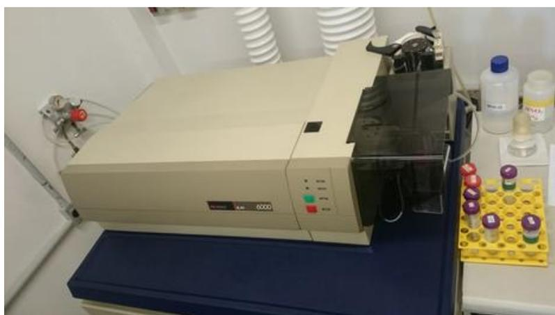
**Figure 3: ICP-MS Elan 6000 model, Perkin Elmer, used for the analysis**
