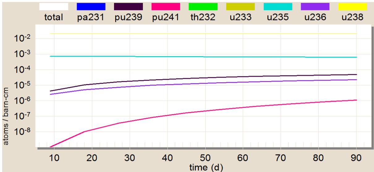
**Figure 3 - Isotopes generated by the burnup of Angra II with 0% of ThO<sub>2</sub>.**
