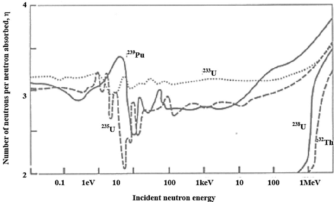
**Figure 2 - Neutron yield per neutron absorbed [04].**
