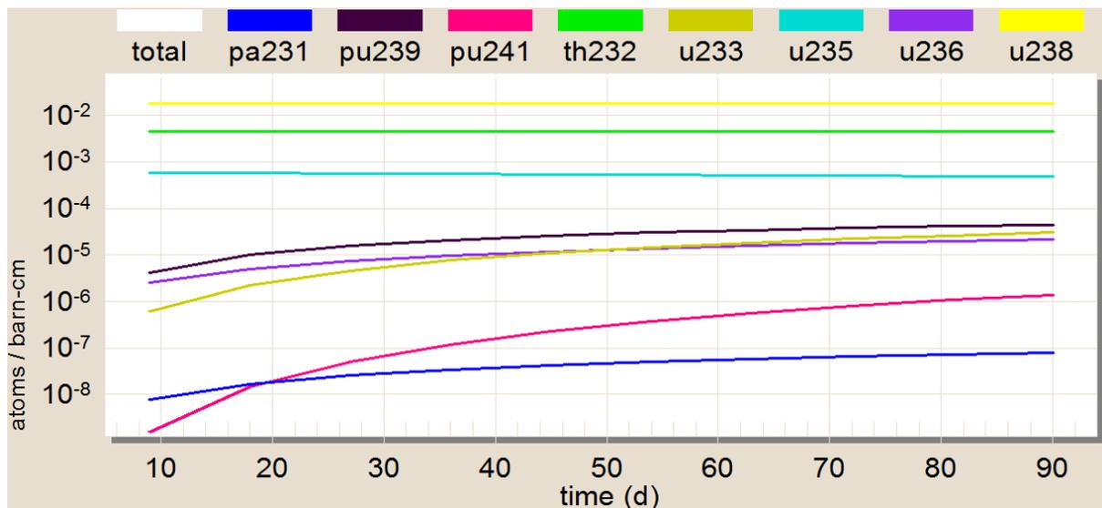
**Figure 5 - Isotopes generated by the burnup of Angra II with 20% of ThO<sub>2</sub>.**
