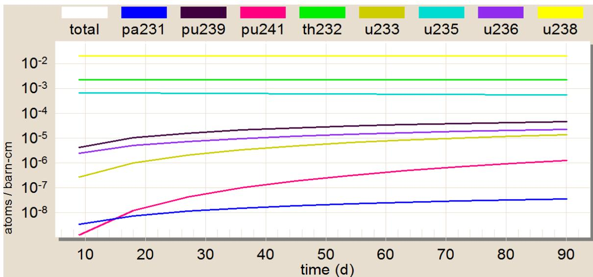
**Figure 4 - Isotopes generated by the burnup of Angra II with 10% of ThO<sub>2</sub>.**
