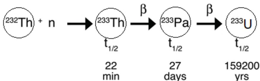
**Figure 1 -  $^{232}\text{Th}$  fertilization process and transmutation into  $^{233}\text{U}$  [02].**
