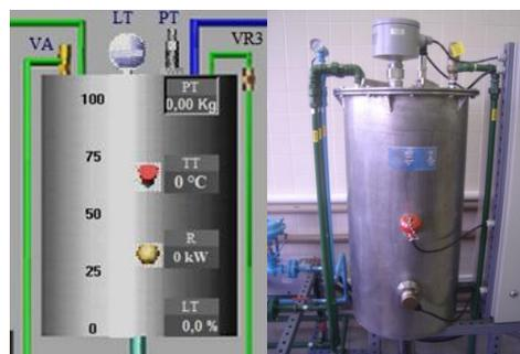
Figure 3: Pressure Vessel used in experiments.
