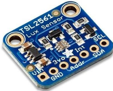
Figure 5: TSL2561 Digital Luminosity Sensor [10].
