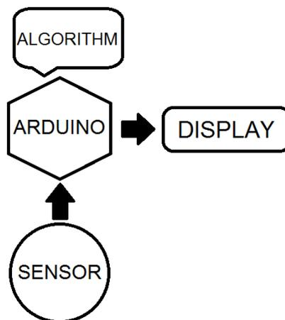
Figure 7: Block diagram for the microcontroller proposal.
