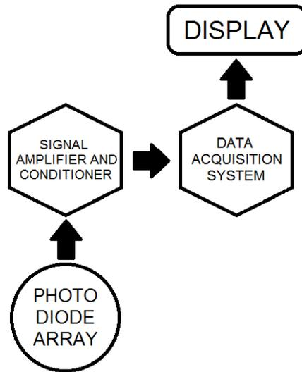
**Figure 3: Block diagram for the photo diode proposal.**
