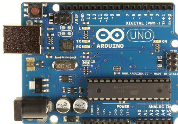
**Figure 4: Arduino UNO board [9].**
