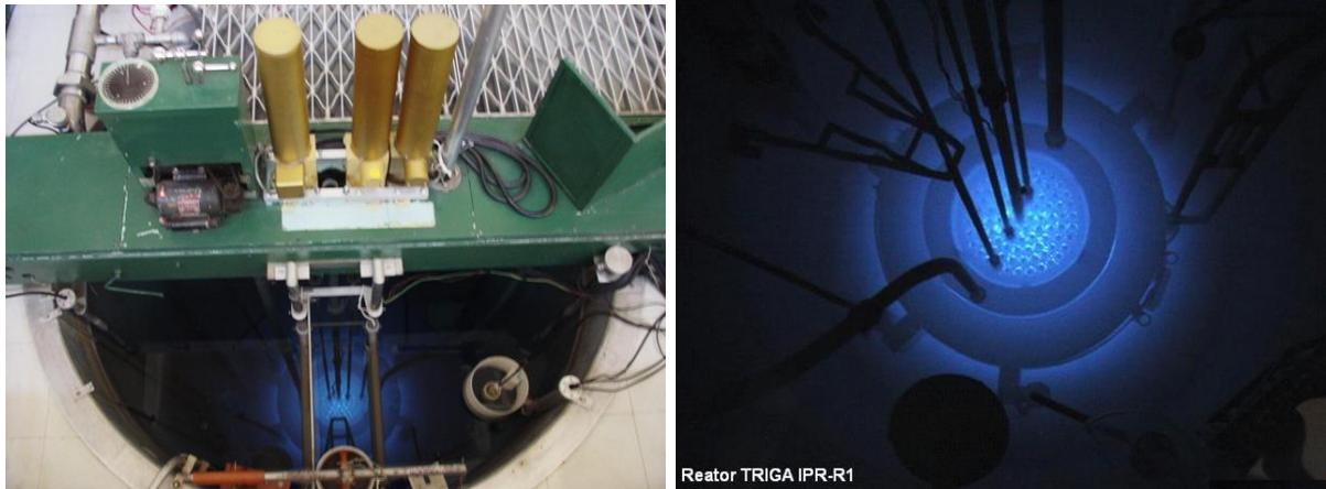
**Figure 1: Cherenkov Radiation in the IPR-R1 Research Reactor Pool [3].**
