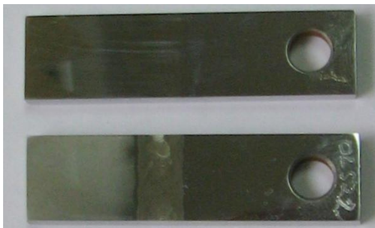
Figure 2 The aspect of dissimilar welds between 52.2k carbon steel and 420 martensitic stainless steels
