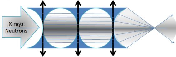
Fig. 1. Schematic view of compound refractive lens.
