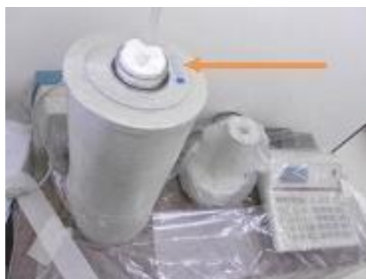
Figure 4: Capintec15W. Emphasis on sample holder for the measures.
