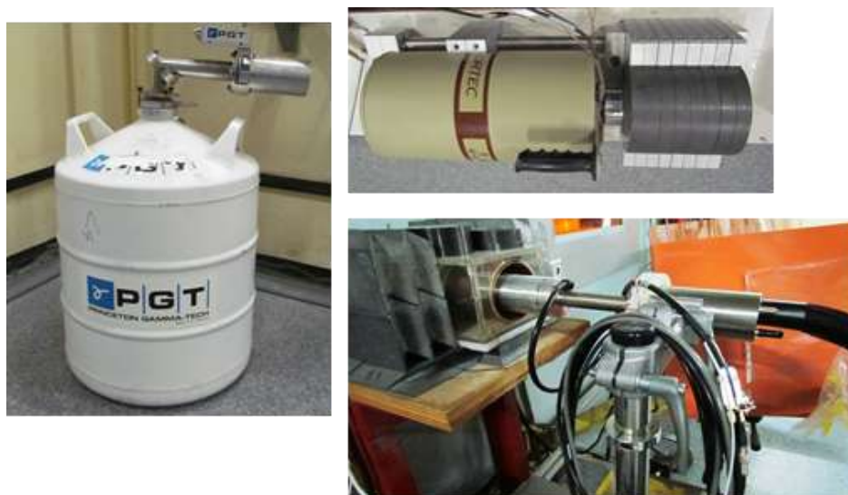
Fig. 1. PGT – IGC 12(1986)/ORTEC NOMAD PLUS (1998)/ORTEC GEM 30 P4-70 (2014) - HP Ge Detectors
