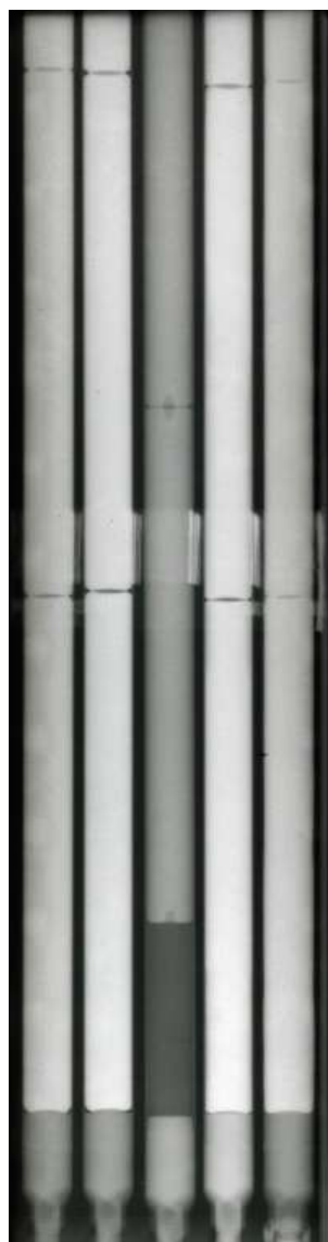
Image 9 – For spent TRIGA-HEU, fresh TRIGA-HEU, standard with iron pellets, fresh TRIGA-LEU, spent TRIGA-LEU image obtained with dysprosium
