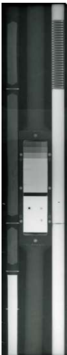
Image 7 – For dimensional standard, IQI and fresh TRIGA-LEU nuclear fuel image obtained with dysprosium
