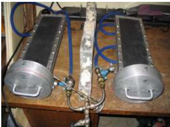
Fig. 5 - Vacuum chambers for image transfer from metallic foils to radiographic films
