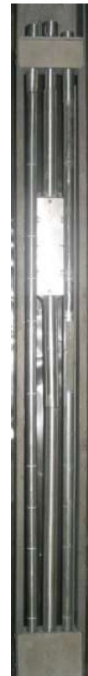
Fig. 2 - Special holder for nuclear fuel elements with IQI (in middle) and two other standards
