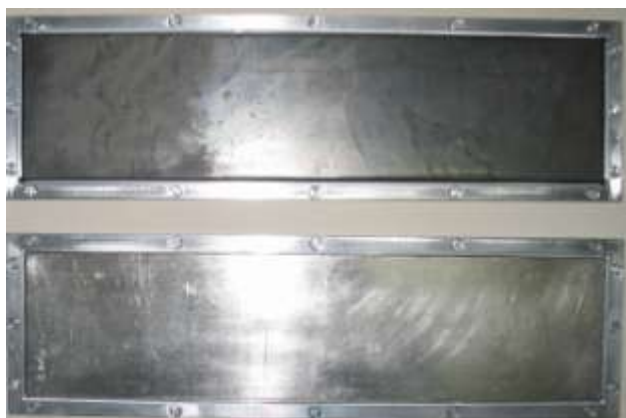
Fig. 3 - Holders for dysprosium foil (top) and indium foil (bottom)
