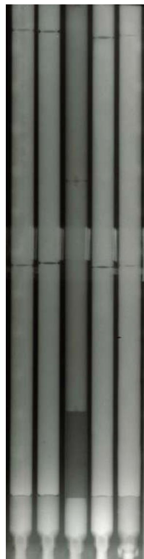
Image 10 – For spent TRIGA-HEU, fresh TRIGA-HEU, standard with iron pellets, fresh TRIGA-LEU, spent TRIGA-LEU image obtained with indium
