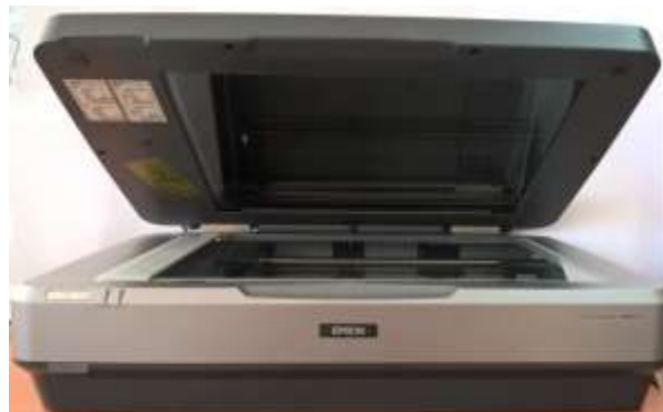
Fig. 6 - EPSON EXPRESSION 10000XL professional scanner for radiographic films
