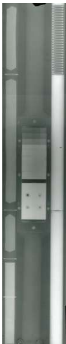
Image 8 – For dimensional standard, IQI and fresh TRIGA-LEU nuclear fuel image obtained with indium
