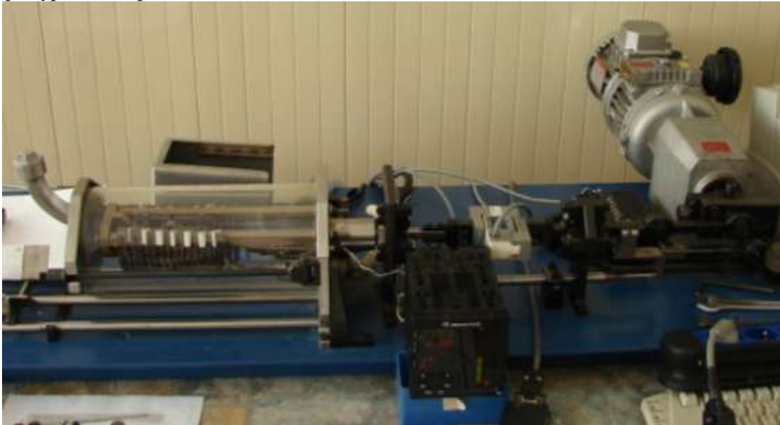
Fig.1. The equipment used for simulated power cycling fatigue
