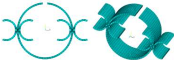
Fig.4. Modelling of “C-ring” samples using ANSYS
