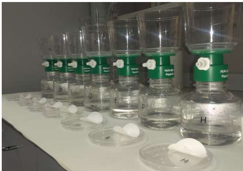
Fig. 5 Solution filtering on filter paper with porosity of 0.2 \mu\text{m}
