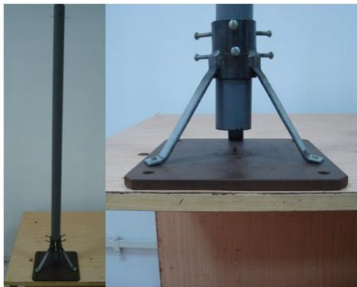
Fig.4. The device for the puncture test
