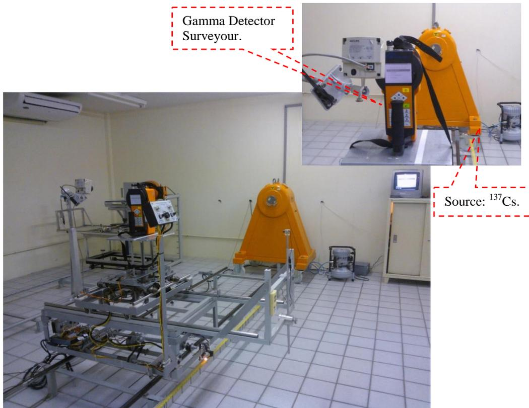
**Figure 3: Arrangement to be adopted for gamma detector calibration.**
