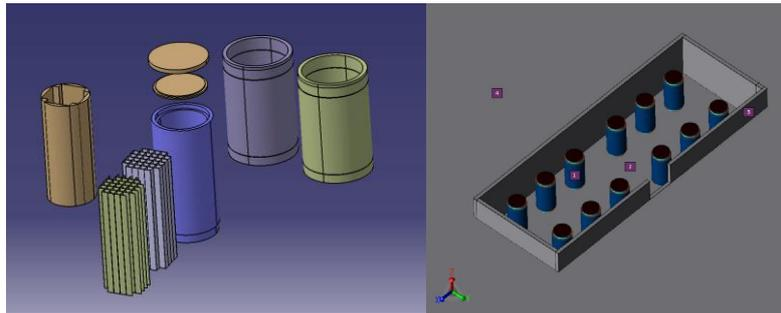
**Figure 16: Spent fuel casks elements and matrix configuration**
