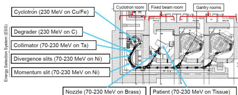
**Figure 14: Scheme of a proton-therapy facility**
