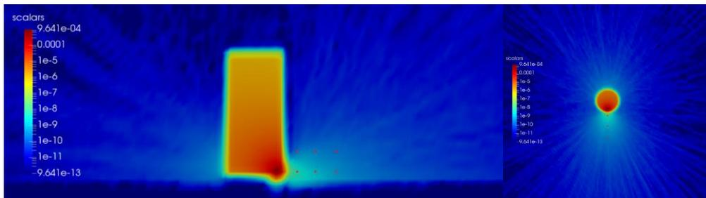
**Figure 17: Near field dose rate due to one cask**
