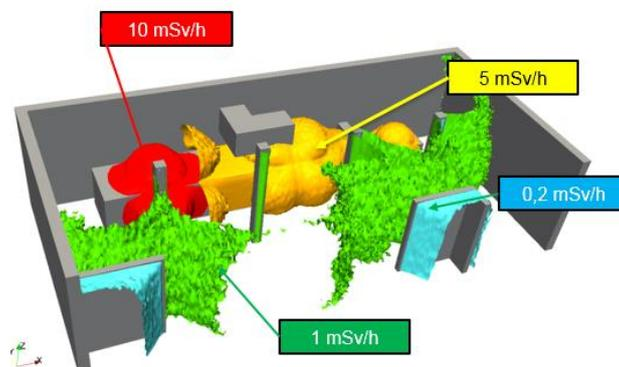
**Figure 14: Filtering Units iso-surface dose rates**
