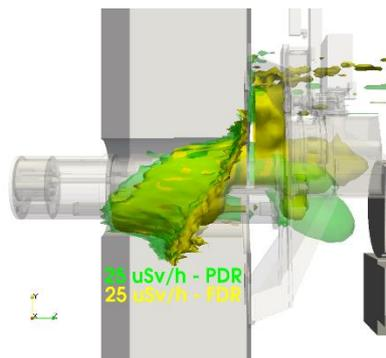
**Figure 9:  $25 \mu\text{Sv/h}$  Dose Rate 3D contour plot comparison between Final Design (FDR) and Preliminary Design (PDR) for Nominal situation.**
