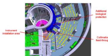
**Figure 1: JHR pool Collimator.**
