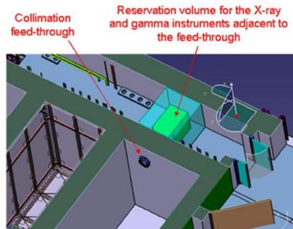
**Figure 2: Irradiated Components Storage pool Collimator.**
