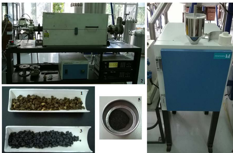
Figure 1: (1) macauba endocarp pre-pyrolysis; (2) pyrolysis reactor; (3) biochar; (4) cutting mill; (5) ground biochar.
