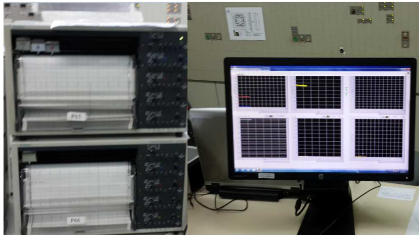
Figure 2: Strip chart of old system acquisition and Front Panel of the new system, during the cycle 13 physical tests.
