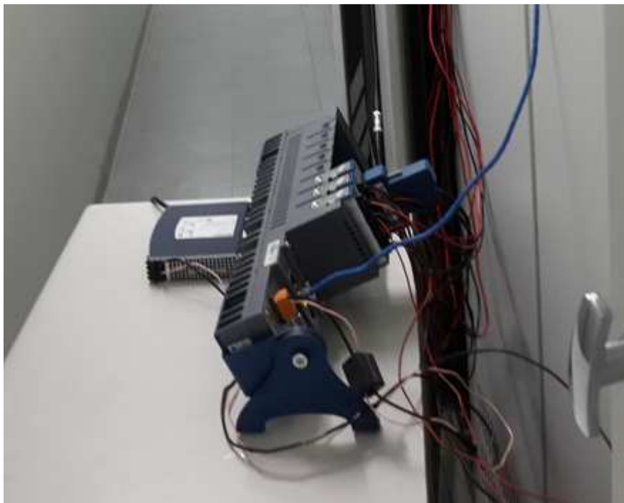
Figure 1: CWX Panel of test computer - cRIO 9082 controller in use during cycle 13 physical tests.
