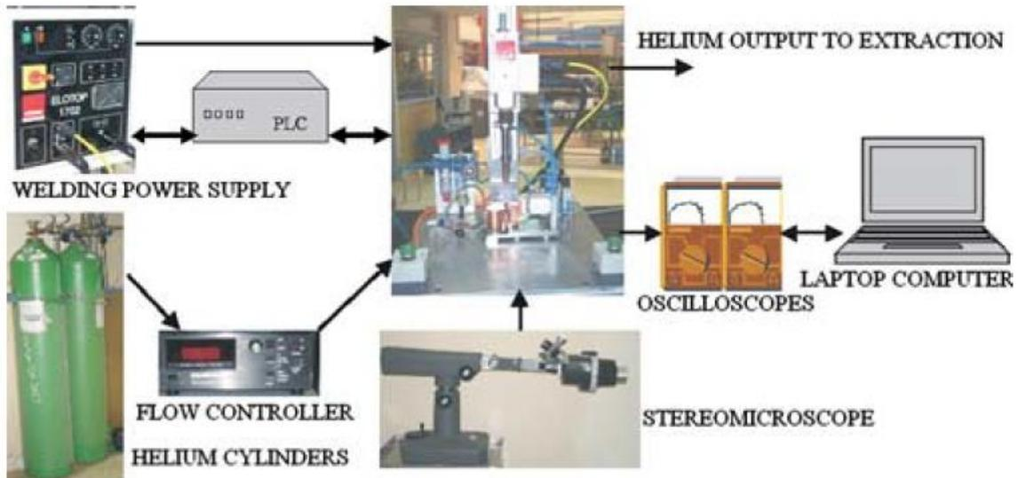
**Figure 1: Welding system diagram [2].**
