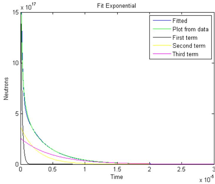
**Figure 2: Plot with the adjusted function, compared with the data and with each one of the terms of the exponential.**
