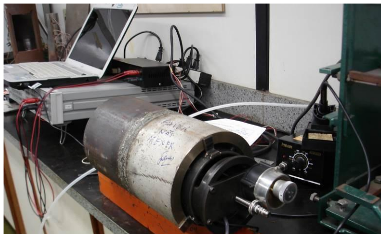
Figure 4: The equipment to measure strains inner surface the pipes installed inside the welded pipe.
