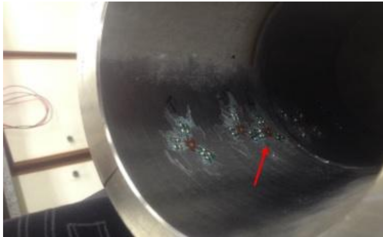
Figure 3: Positioning of the strain gages rosette type used in internal residual stress measurements.
