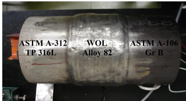
Figure 5. The weld overlay on the dissimilar welded pipe.
