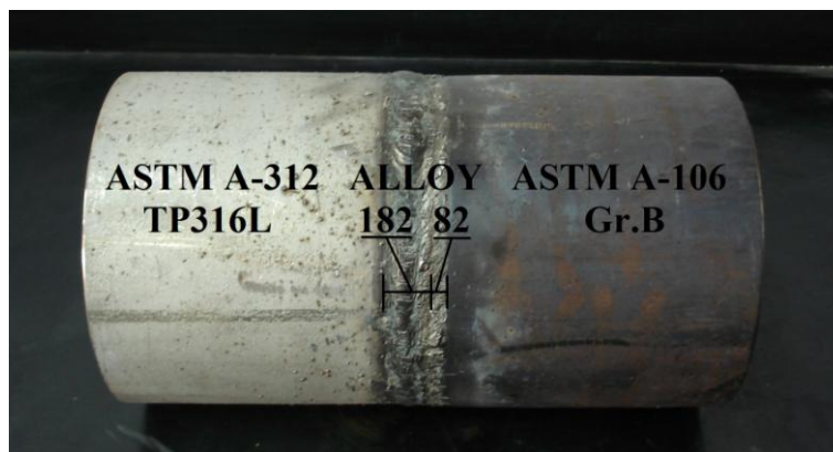
Figure 2: Dissimilar welded pipes, austenitic stainless steel (ASTM A-312 TP316L) carbon steel (ASTM A-106 Gr B) and filler metals (Alloy 82 and 182).
