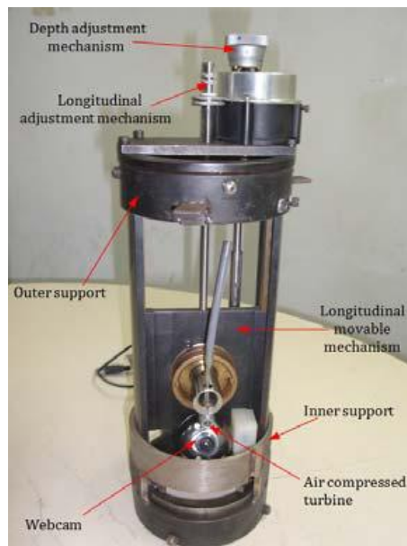
Figure 1: Developed equipment to assist measuring residual stresses inner wall pipes by hole-drilling method [23].
