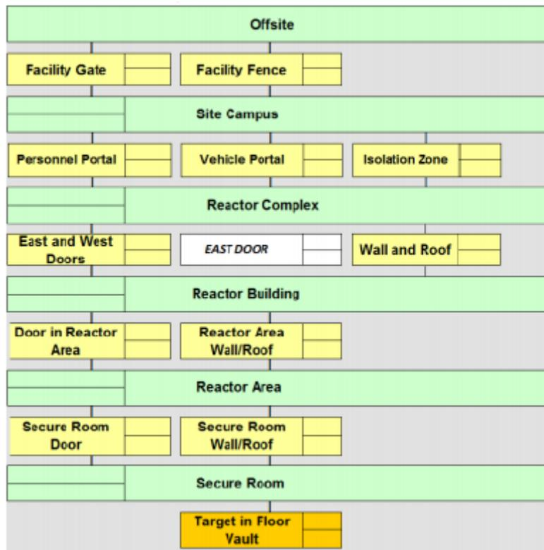
**Figure 2: ASD for reactor building – fresh fuel vault target.**
