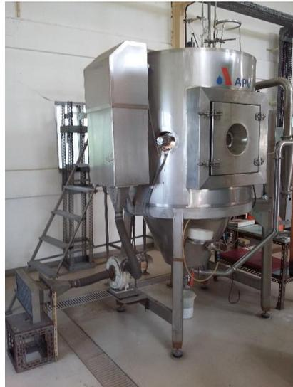
**Figure 3: Spray Dryer APV – IEN-RJ.**
