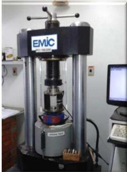
**Figure 2: Compressive Strength Test**
